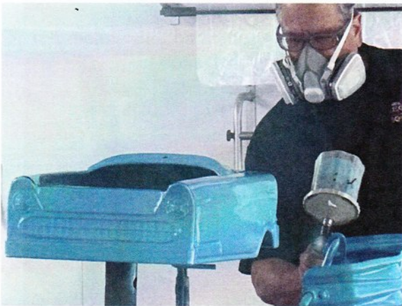
Tee Bird blue gets applied to the body and other parts (left).
